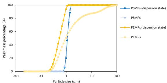
Fig.1 Particle-size distribution of PSMPs and PEMPs. A dispersant and ultrasound were used to measure the particle size of MPs in the dispersed state.
