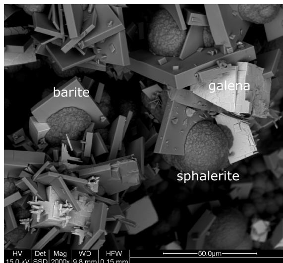
Fig. 1 A backscattered electron image of hydrothermally synthesized sphalerite, galena and barite.
