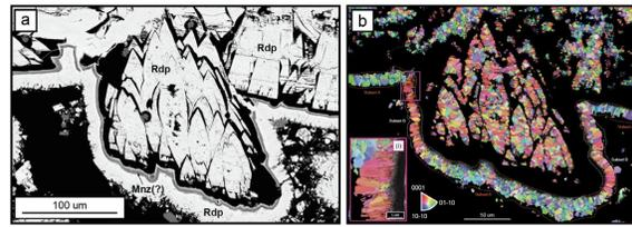
**Figure 1:** Petrographic analysis of dissolution pit preservation through secondary rhabdophane precipitation by: a) SEM imaging (rhabdophane in white, monazite(?) in grey, void space in black), and; b) EBSD. Note both the complete destruction of the primary mineral, and the two preferential and orthogonal orientations of rhabdophane along its 0001 axis (red) and 01-10/10-10 axes (blue, green).
