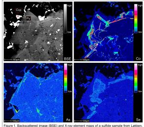
Figure 1. Backscattered image (BSE) and X-ray element maps of a sulfide sample from Løkken, Norway illustrating growth zones of various cobalt, arsenic and selenium concentrations. Py, pyrite; Ccp, chalcopyrite.
