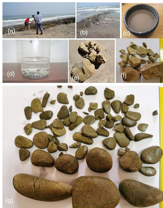
Figs.1a-g. (a) spreading rocks on the beach. (b) Dunite in wood box. (c) Dunite after Tumbling. (d) Carbonate precipitation in beaker after heating and rotation for 6 months. (e-f) Dunite samples used for spreading on the beach and in tumbling. (g) Dunite samples after 3 years of beach surfing.
