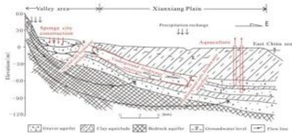
Figure 1 Schematic diagram of building underground freshwater reservoir in the 1 st confined aquifer
