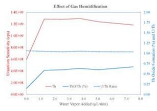
Optimal water vapor addition conditions of 1  $\mu$ Lmin<sup>-1</sup> are used to evaluate trace metal quantification using LA-ICPMS. We compare trace metal results for reference materials over a wide range of matracies.
