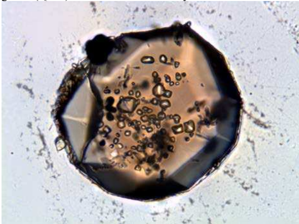
Figure 1. Transmitted light photograph of a garnet crystal containing quartz inclusions grown in an experiment performed at 2.0 GPa and 800°C. At room conditions, average inclusion pressure is 0.82 GPa. Garnet is 100 \mu\text{m} across. Photo is a composite of five stacked images.
