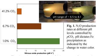
The data shown is based on 24 hour runs of an anoxic reactor and linear regression of the  $N_2O$  headspace determined by IR spectroscopy. We will further present results from experiments with magnetite derived from *Magnetospirillum* cultures as well as FeOOH precipitates produced by photooxidation. Our work can help to better understand the significance of  $N_2O$  in the anoxic Archaean, and complement reaction rates derived from microbial denitrification.
