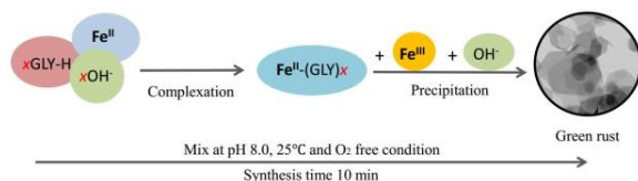
Figure 1: Schematic diagram of GRs synthesis in presence of glycine, Fe II and Fe III salt solutions.
