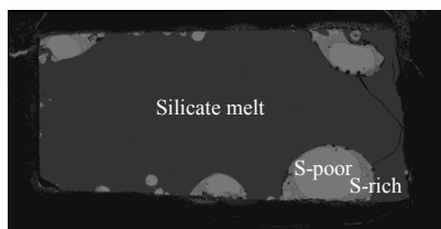
Figure 1. Scanning electron microscope composition images of the quenched samples at 1GPa, 1600°C. Two immiscible liquids (S-rich and S-poor melts) and one homogenous silicate melt are the run products.
