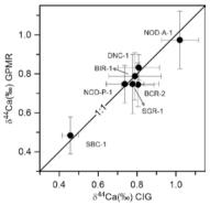
**Fig. 1**. Comparison of Ca isotopic compositions of USGS reference materials measured in CIG and GPMR. Error bars represent 2 standard deviations (2s) of each measurement.
