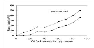
It was found that removal of straight line continua over the 1 and 2  $\mu$ m absorption bands was sufficient to recover band centers, required for determining LCP composition.
