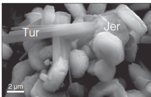
Figure 1: SEM image of olenitic tourmaline (Tur) that forms from jeremejevite (Jer) as a precursor phase after 0.5 h.
