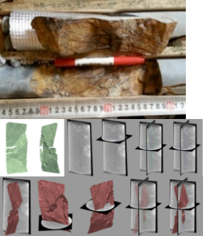
Fig.1. Fractured rock sample and the result of XMT for core sample with fractures
