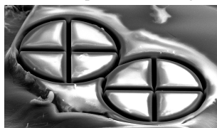
Fig. 1: Secondary electron image of a single-crystal ringwoodite FIB-cut into divided circles, \varnothing=120\ \mu\text{m} .
