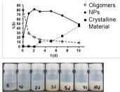
Figure1. Zeolite beta crystallization from clear solution monitored by <sup>29</sup>Si NMR.
