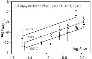
Figure 1. The dependence of Nd fugasity in gas with water pressure.
