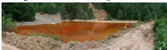
Figure 1. Several views from Kuvarshan mine: (a) discharges enriched with sulfate salts (b) precipitation of sulfate minerals (c) acidic pond developed in mine waste
