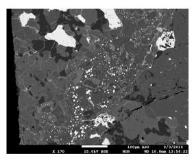
**Results and Discussion:** Unique textures of entrained host-fragments were found in melt vein in several GRV chondrites under high-resolution BSE imaging (see Fig above). Preliminary result show abundant partial solid-stated transformation of olivine and pyroxene, and Fe-Mg diffusion. Further results of Raman spectra may be obtained to identify the phases. More discussion will be available in the meeting.
