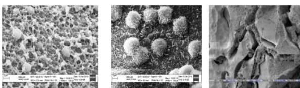
Fig 1: Back scattered SEM image of sodium and barium borosilicate glass and obsidian treated in hydrothermal-like conditions.
