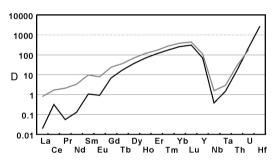
Zircon/rock partition coefficients (D) obtained in this study (black line) and comparative value (grey line, L.V.S. Nardi *et al*, 2013)
