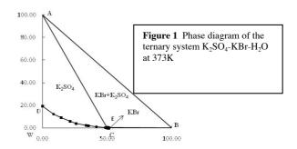
(AED field) in the phase diagram is obviously bigger than that of KBr (BEC field).
