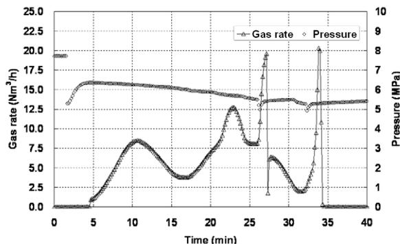
**Figure 1:** Time-dependent variations of gas production rate and well pressure.
