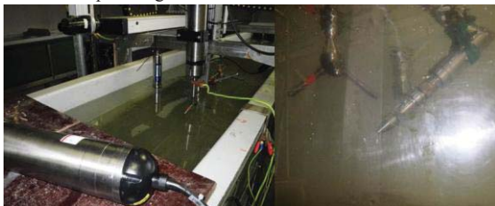
Figure 1: The flume Eddy Covariance deployment (Sept. 2011) showing sensor set-up (velocimeter, left and microelectrode, right).
