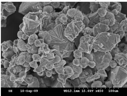
Figure 1 SEM images of carbonate minerals with different morphologies at the 55-th day by using SN-1 strain
