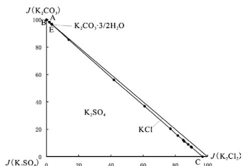
**Figure 1.** Metastable phase diagram of the quaternary system  $\text{K}^+/\text{Cl}^-$ ,  $\text{CO}_3^{2-}$ ,  $\text{SO}_4^{2-}$ - $\text{H}_2\text{O}$  at 273.15 K
