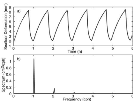
**Figure 1:** a) Modeled GSD and b) the spectrum of the modeled GSD signal above the TAG hydrothermal field.
