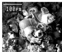
Figure 1: Evidence of gas evolution at DU metal surface. Figure 2: Fungal hyphae on DU metal surface.
