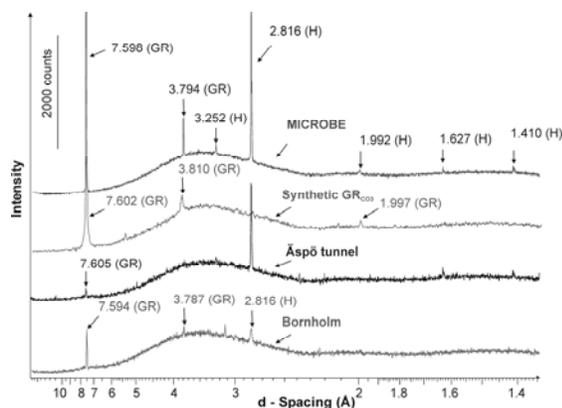
XRD patterns from the natural samples and a synthetic GR<sub>CO3</sub>. The peaks representing reflections from the basal plane have d-spacings ~7.6 and ~3.8 Å are characteristic for the carbonate form of green rust. H marks halite reflections (from [1]).
