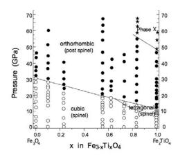
The solid solutions with  $0.734 \le x \le 1.0$  show the transition from the cubic to the tetragonal spinel. The transition pressures are 12 GPa at x=0.734 and 8 GPa at x=1.0. This transition is due to Jahn-Teller effect of Fe<sup>2+</sup> (3d<sup>6</sup>). The tetragonal phase is not observed in the samples with x<0.624. An unknown phase at x=1.0 was found at 48 GPa.
