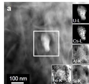
**Figure 1:** HAADF-STEM of Cs-U-phase with the elemental maps.
