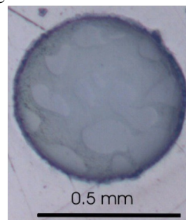
Figure 1: Calcite sphere grown in an acrylamide cryogel (gelation at -20°C).
