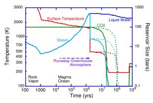
A cartoon history of water, temperature, and carbon dioxide in the aftermath of the moon-forming impact. How long it stays hot depends on how long it takes to scrub the  $CO_2$  out of the atmosphere.
