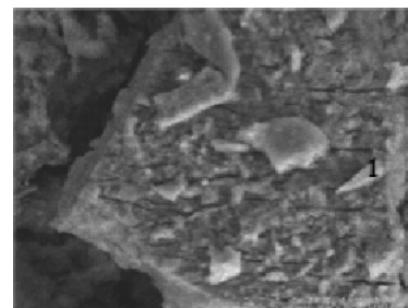
Apatite II™ collected from the PRB after 3 years showing sphalerite on surface
