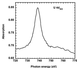
NEXAFS spectrum collected at the U 4d<sub>5/2</sub> edge from a 35 nm edge region of a UO<sub>2</sub> particle.
