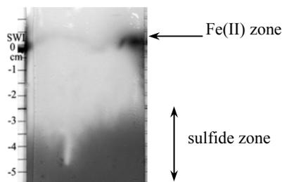
For 1D investigations we have developed a double-side probe using a DGT for one face and a DET for the second face in order to compare Cd measurements with minors components, such as Fe and Mn, minimizing spatial effects in heterogeneous sediment. Trace elements are analyzed by ICP-AES, ICP-MS and GF-AAS. The DGT face can be analyzed by LA-ICP-MS to get 2D distribution of trace metals.
