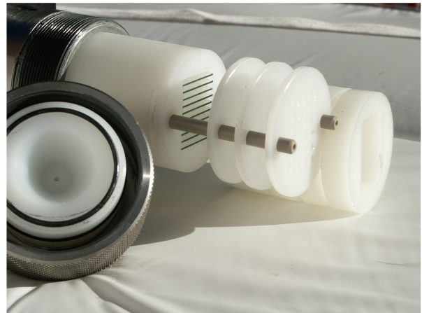
Figure: Pressure resistant laminar flow cell for investigations of in situ biofilm formation. Three flow diffusers are installed before and after the pile of laminar surfaces for growth.
