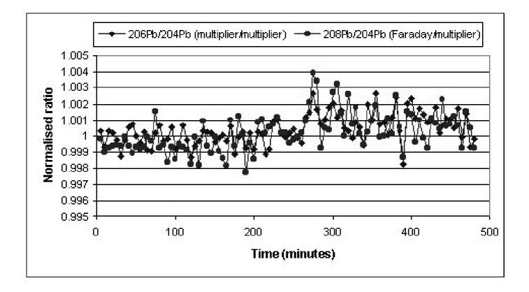
Figure 1: Isotope ratio stability of the VG Axiom Multiple Multiplier system
