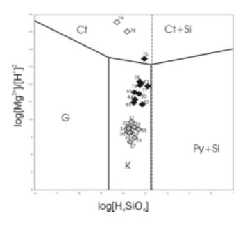
Figure 1.: Activity diagram at 25 °C and 1 bar for the system MgO-SiO<sub>2</sub>-H<sub>2</sub>O. The black diamonds are spring waters without gas phase. The gray diamonds are waters with  $CO_2$ -dominant gas phase. The white diamonds are different by origin (one from the Lake Balaton, and one from the Bels Z337;-tó).
